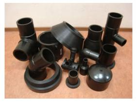
Production of fittings comprises mitre cutting of polyethylene pipes of predetermined size and welding of workpieces by butt welding. The fittings are used during installation of polyethylene pipes for water and sanitation from 50 to 630 mm.
